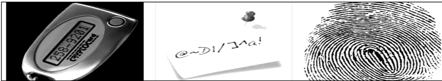
Fig. 3.10 : What you have (Token), what you know (password/PIN) and who you are (Biometric)
